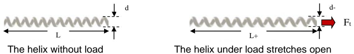
Figure 4 – How the helix responds under tension.
