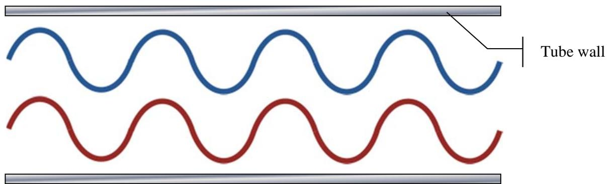
Figure 6 – Fibers inside a loose tube
