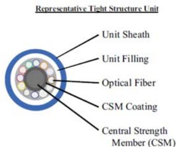
Figure 8 – A typical tight buffer tube.
