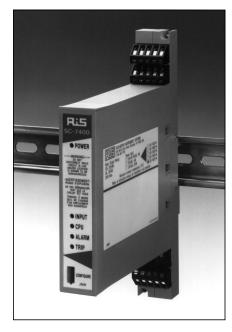
The SC-7400 is an intelligent, universal input signal conditioner/alarm trip that isolates and transmits the status of process signals on a single control loop basis. It handles a variety of temperature and process inputs and offers combinations of analog and relay contact outputs.
